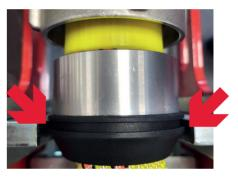
The notch of the outer ring must be placed in the form.
