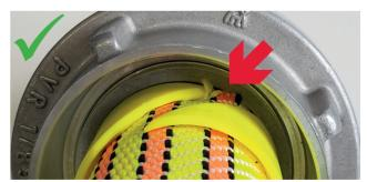
The notch of the inner ring must be on the opposite side of the
