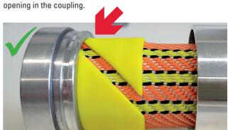
The shoulder of the inner ring must be pushed completely into the nozzle by hand with a positive fit before the pressing process (see illustration on the right).
