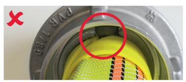
The notch of the inner ring should never be aligned with the opening in the coupling.
