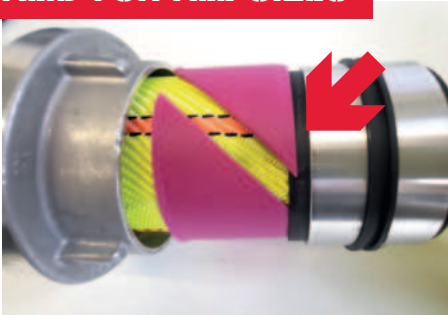
The outer ring must be placed manually next to the inner ring.
