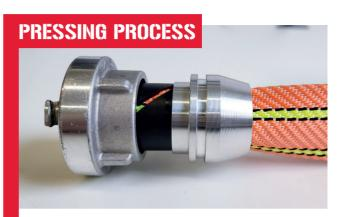
The outer ring must be placed on the inner ring by hand. The inner ring must fit exactly into the outer ring.
